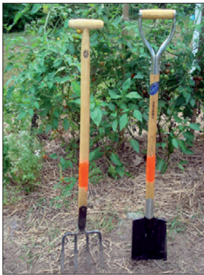
A digging fork (left) with a T-handle and a spade with a D-handle. Photo: Andy Pressman, NCAT
