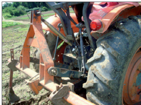
A three-point hitch. Photo: Andy Pressman, NCAT
