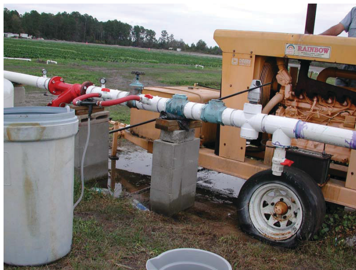
Figure 2. Diesel engines mounted on a trailer offer the greatest flexibility of use.
